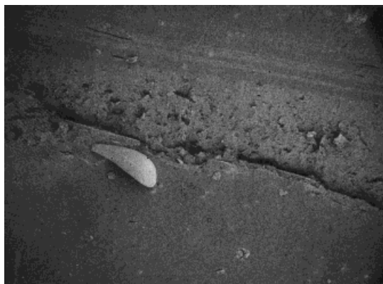
Figure 17 SEM fractography of tensile fractured specimen of EPDM after aging at 100°C (original magnification \times 500 ).
